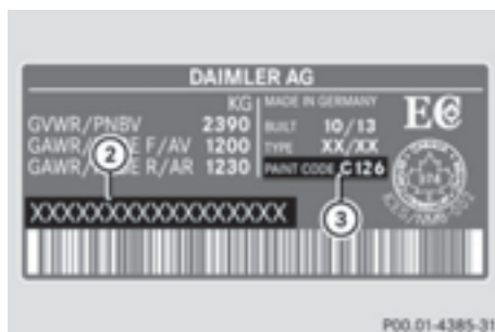
Example: vehicle identification plate (Canada only)
