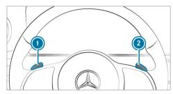
Pull steering wheel paddle shifters ① and ② and hold for half a second.
