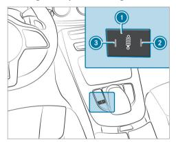
➤ To select the Comfort suspension setting: press button ① repeatedly until indicator lamps ② and ③ go out.
