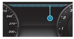
If the engine speed is too high or too low, you cannot change gear using the steering wheel paddle shifters. In this case, segments • light up red.
