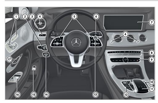
Adjusts the seat electrically Seat ventilation Adjusts the front passenger seat Memory function and memory presets 1 2 3 2 Light switch (3) Driver assistance systems Active Steering Assist Active Lane Keeping Assist Switches off Parking Assist **PARKTRONIC** Depending on the vehicle's equipment, the button may also be at position 12. Head-up Display
